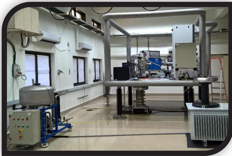
Electron Cyclotron Resonance (ECR) ion source-based low-to-medium energy ion-beam facility at IOP
